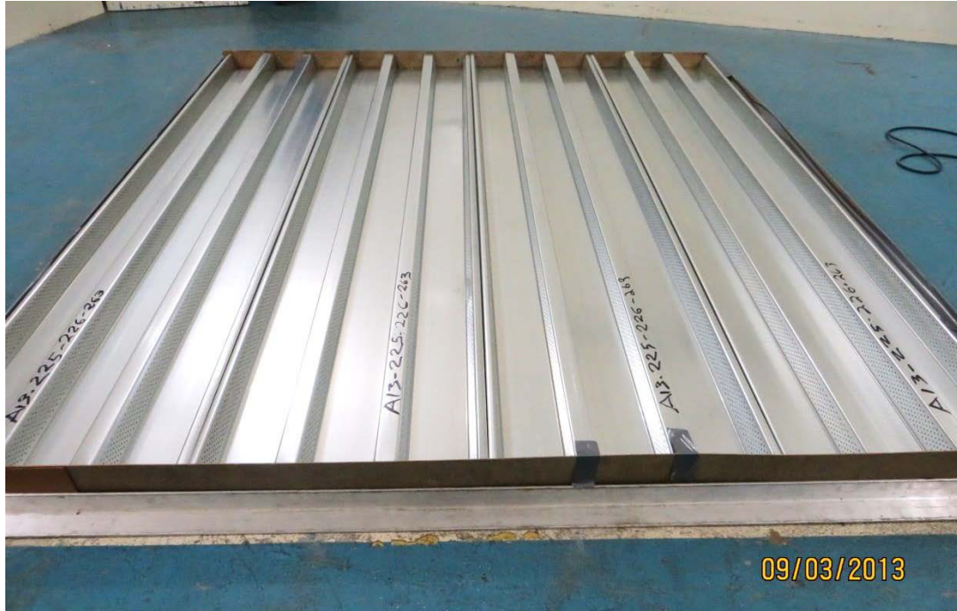
Figure 3 - Specimen mounted in the test chamber.
