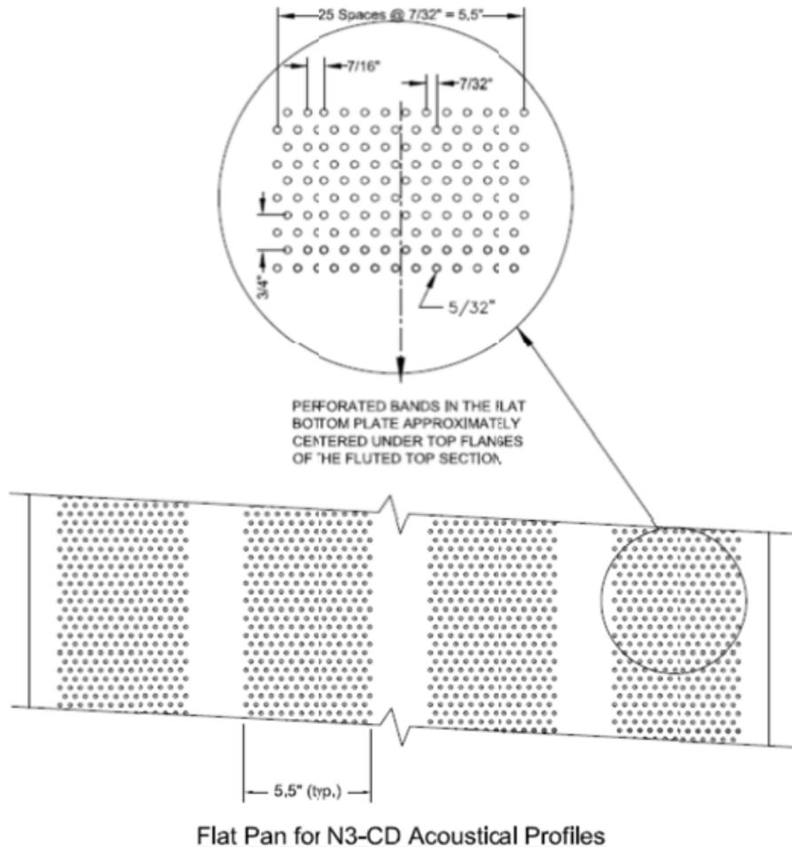
Figure 2 - Acoustical perforation detail (supplied by client).
